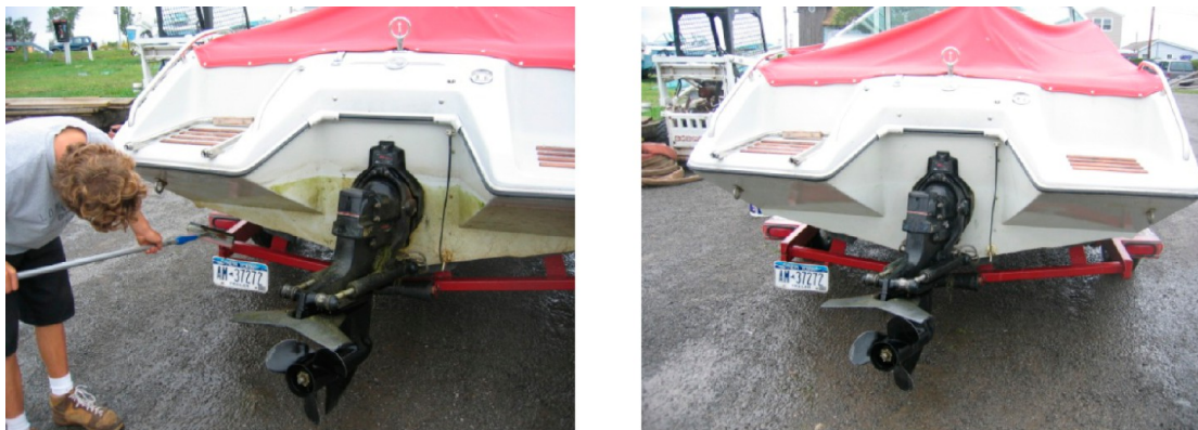
FIGURE 3. The boat whose fiberglass hull was coated with the 1:1 C8/TEOS sol–gel paint after its pulling from the Irondequoit Bay (NY) waters (left) and following mild polishing (right). Reproduced with kind permission of Dr. M. R. Detty.
