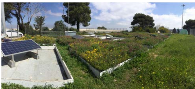
Figure 6. The PV modules on conventional and on green roof tested in 2016 and in 2017 at the University of Haifa (photograph courtesy of Professor Bracha Schindler).
